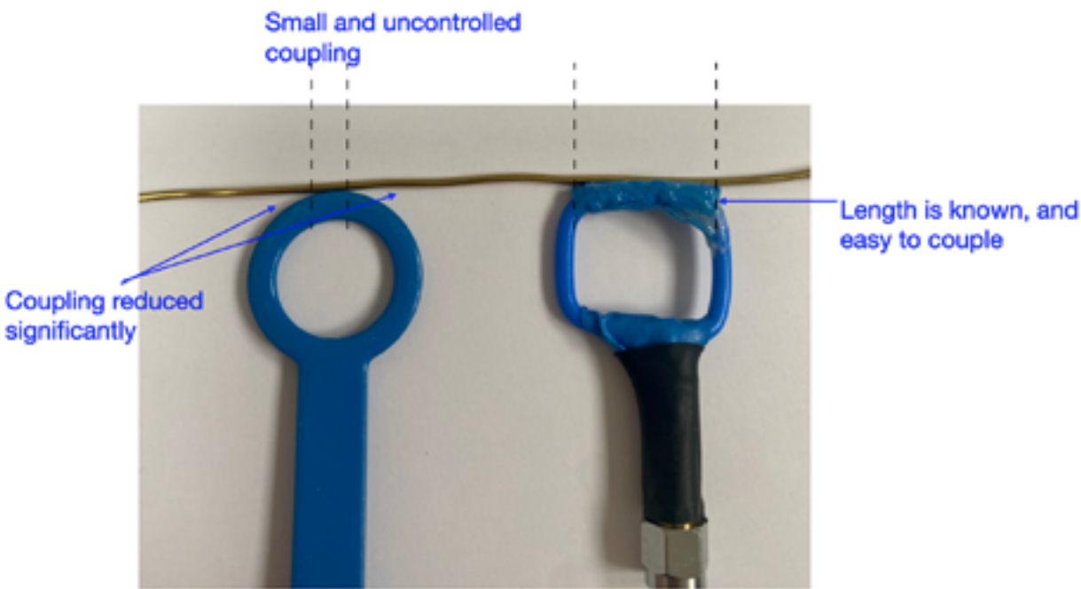
Figure 4 Square shaped vs round shaped magnetic field loop
