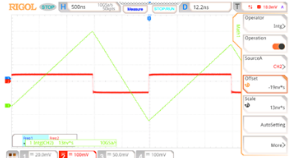
Figure 9 Placing the loop over the inductor gives the induced voltage caused by current going through the inductor. The integration of the waveform gives the inductor current waveform
