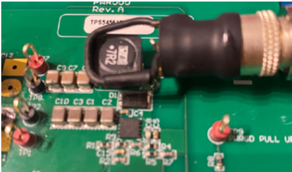
Figure 8 Placing a magnetic field loop horizontally over the PCB and move along the loop until the maximum induced voltage is seen in the oscilloscope
