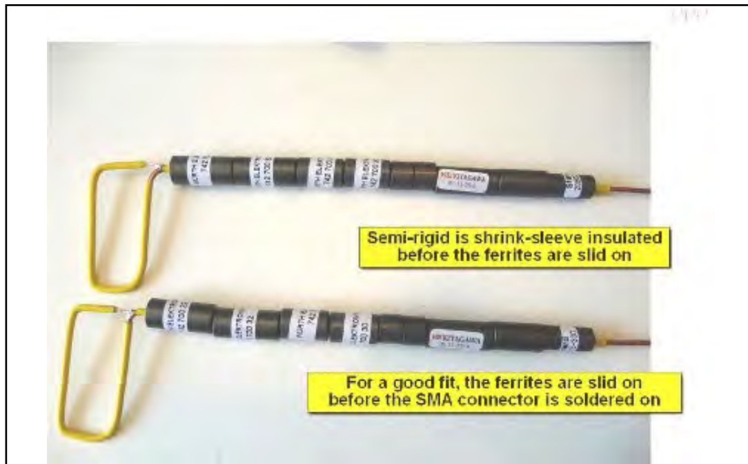
Figure 12 A view of my new probes during a assembly
