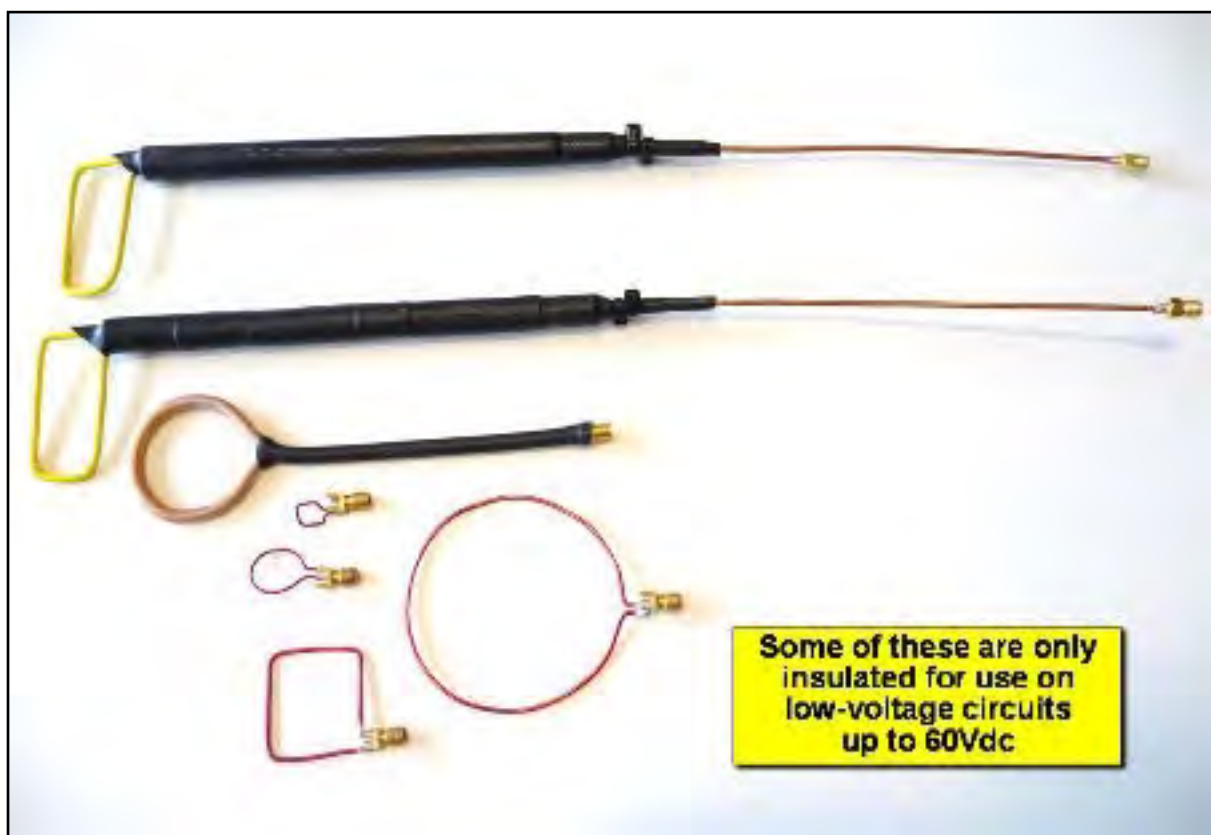
Figure 5 The range of close-field probes that I use (at the time of writing)
