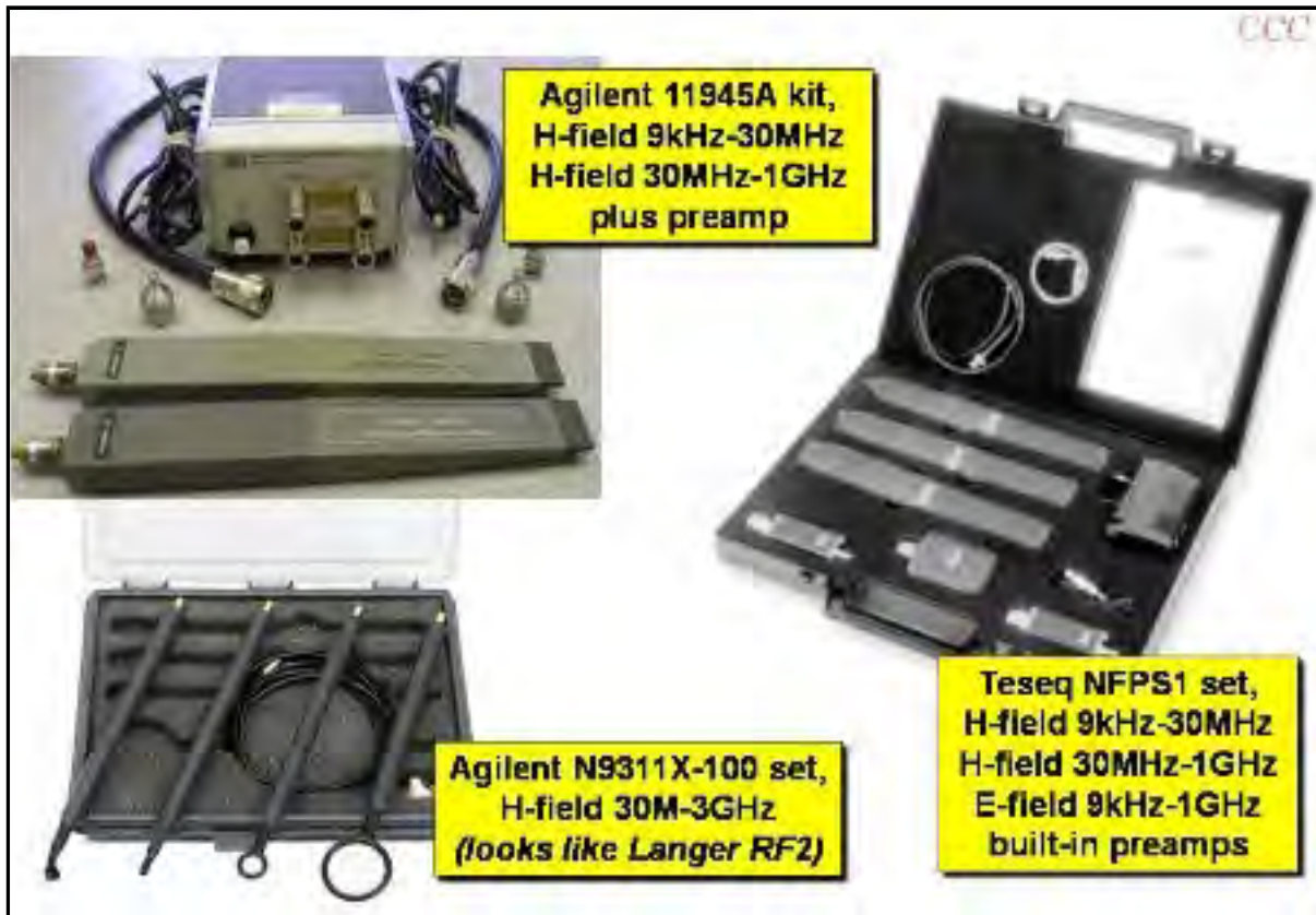
Figure 8 Hewlett-Packard's venerable close-field probes, and currently available ones from Agilent (soon to be renamed Keysight Technologies) and Teseq (which used to be Chase EMC)
