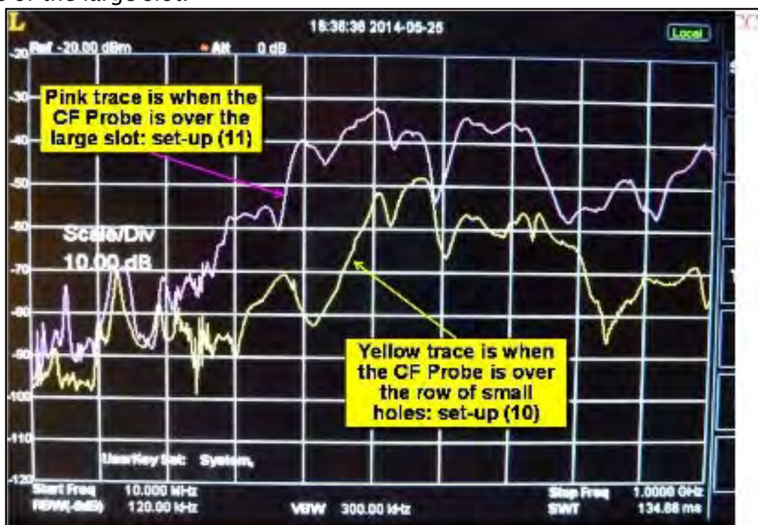
Figure 38 Looking for shielding imperfections with internal illumination - displaying both (10) and (11)
