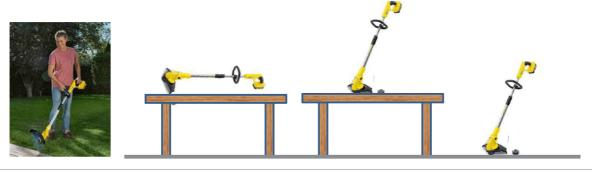
I saw a report from an accredited test house for EMC testing of a line trimmer with no line and no guard lying flat on a table – NOT representative – engineers would argue it is from an accredited test house (see later)
