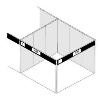
Shell scheme panels are 2.44m High x 1.00m Wide, grey poly weave, velcro compatible.
